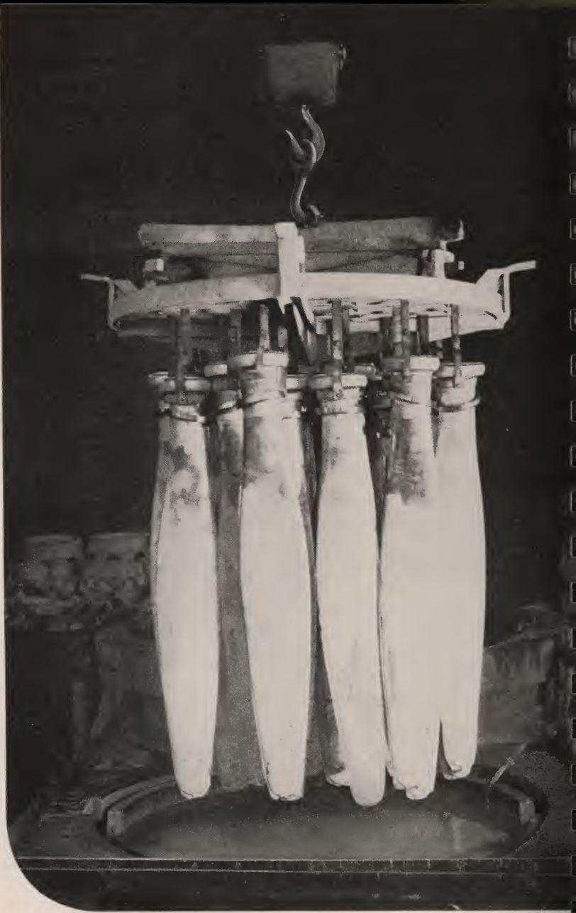
Propeller blades suspended in rack for heat treatment.
